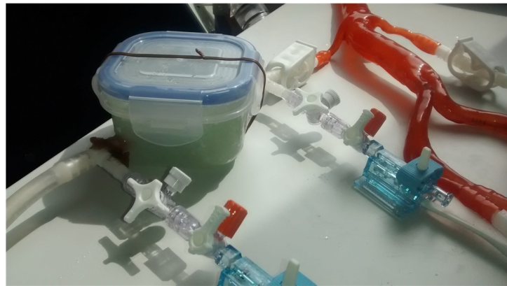
Figure 5.31 The model was extended also of “kidneys” which are simulated as boxes full of small glass balls with diameter less than 1 mm.
